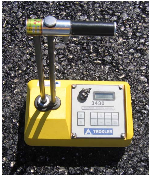
Figure 2. Troxler Model 3430 Nuclear Gauge
