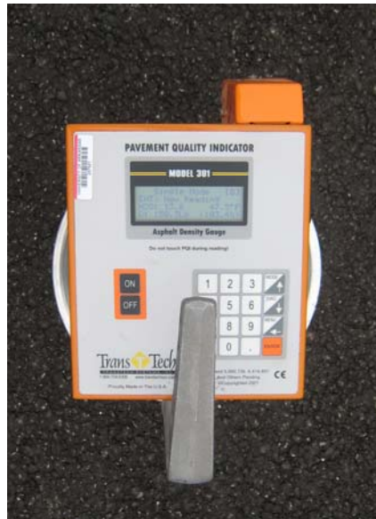
Figure 4. Pavement Quality Indicator™ (PQI) Model 301
