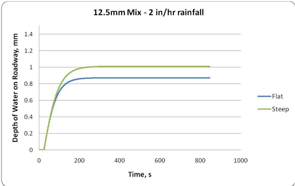
Figure 62. Net Depth of Water on Roadway vs. Time – 12.5mm Mix, Rainfall = 2 in/hr
