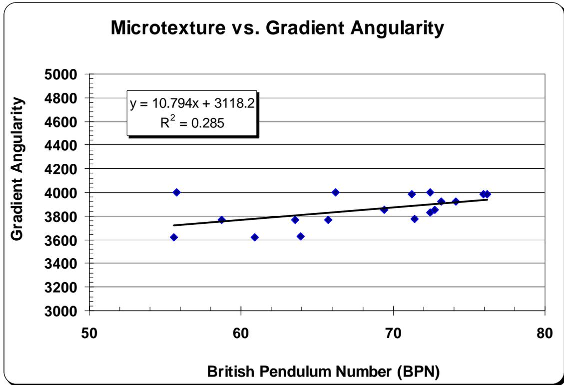
Figure 48. Relationship of Gradient Angularity to Microtexture
