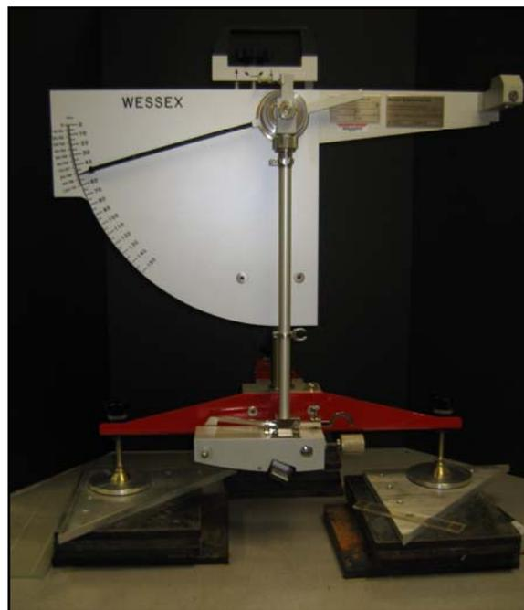
Figure 7. British Pendulum Tester
