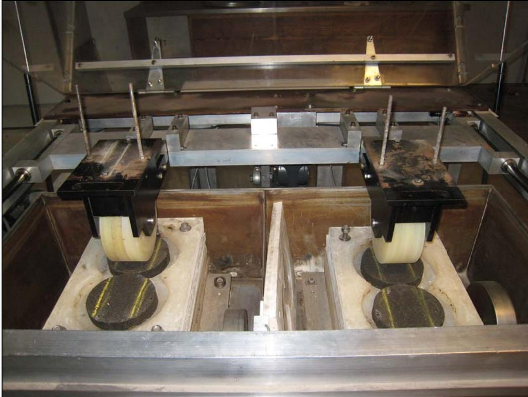
Figure 9. ERSA Device Retrofitted with Conditioning Wheels
