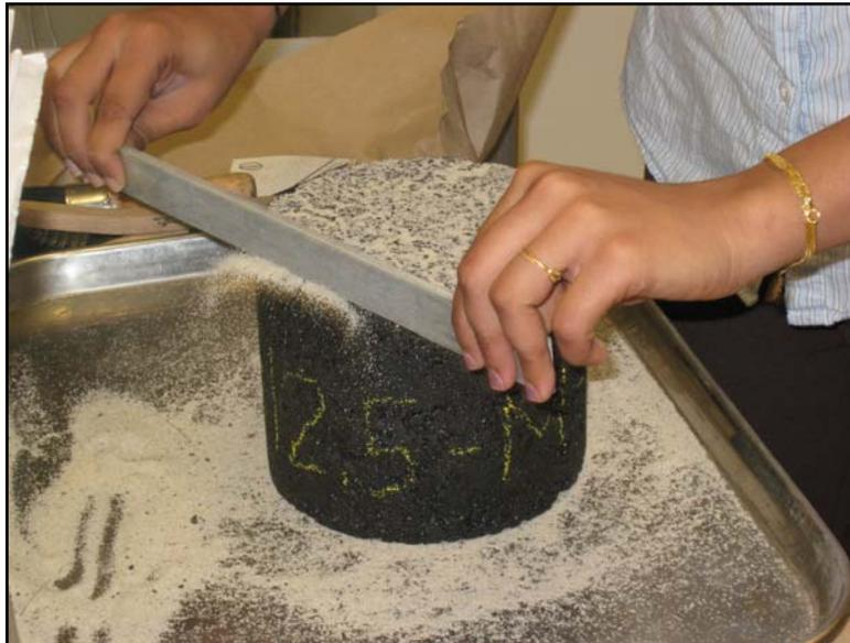
Figure 8. Modified Sand Patch Test
