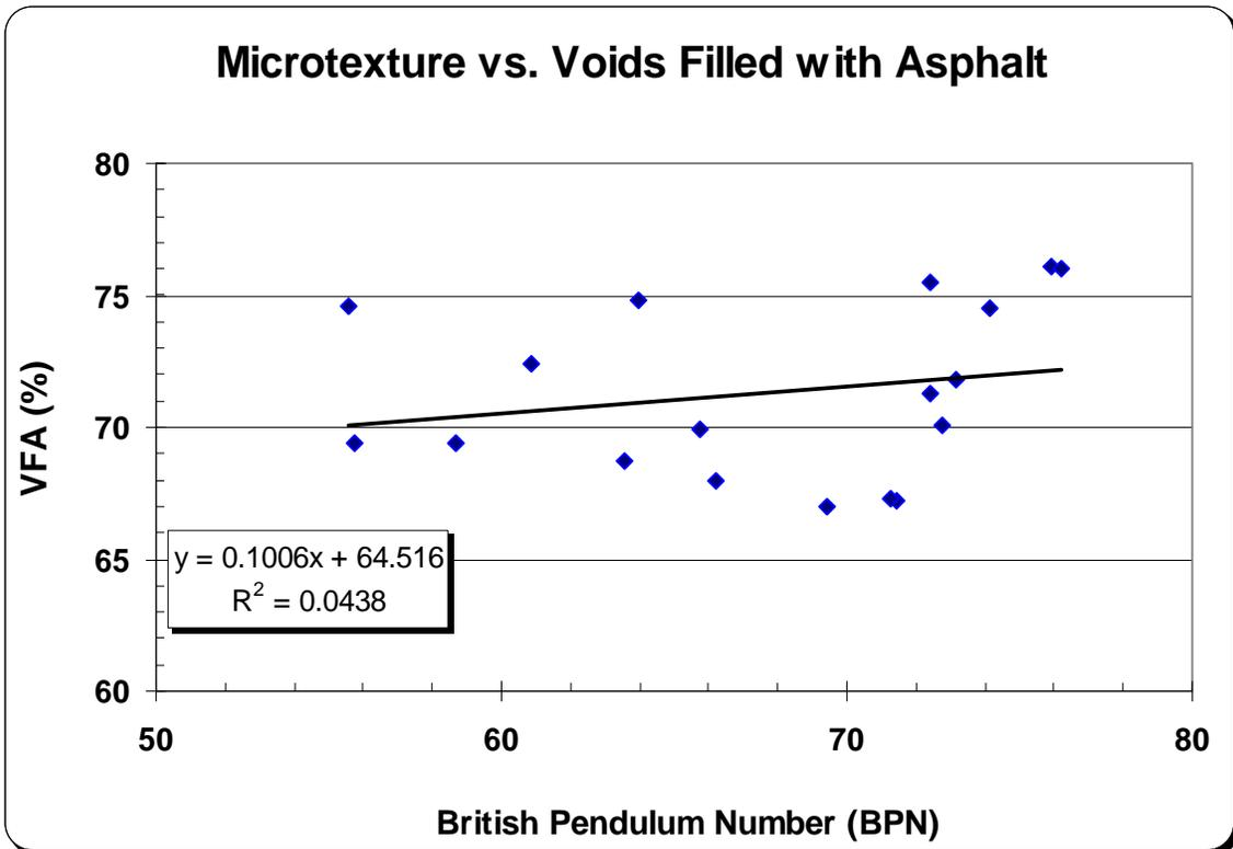
Figure 13. Relationship of Voids Filled with Asphalt (VFA) to Microtexture
