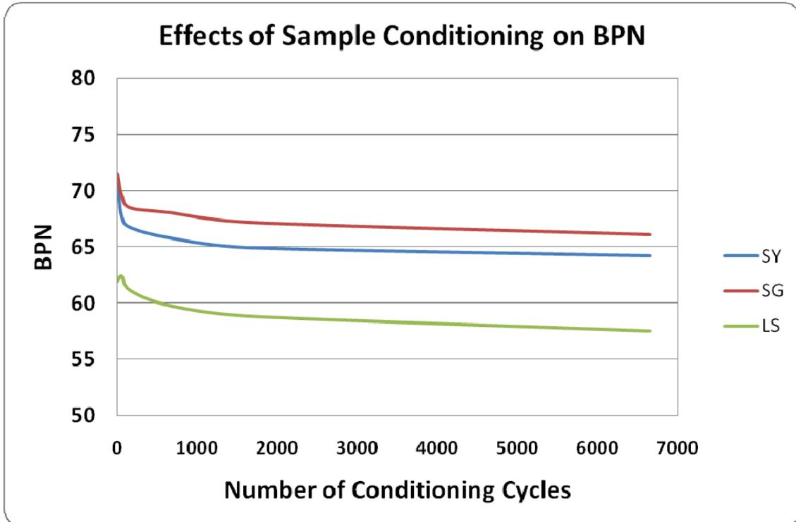
Figure 57. Effect of Specimen Conditioning on Microtexture
