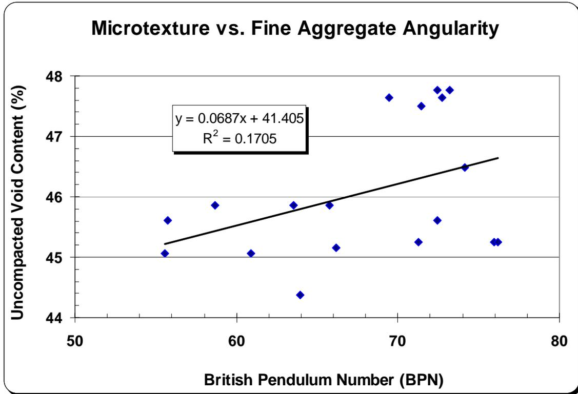
Figure 24. Relationship of Fine Aggregate Angularity to Microtexture
