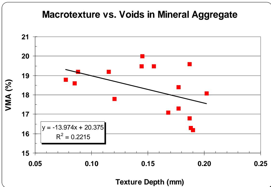
Figure 19. Relationship of Voids in Mineral Aggregate (VMA) to Macrotexture
