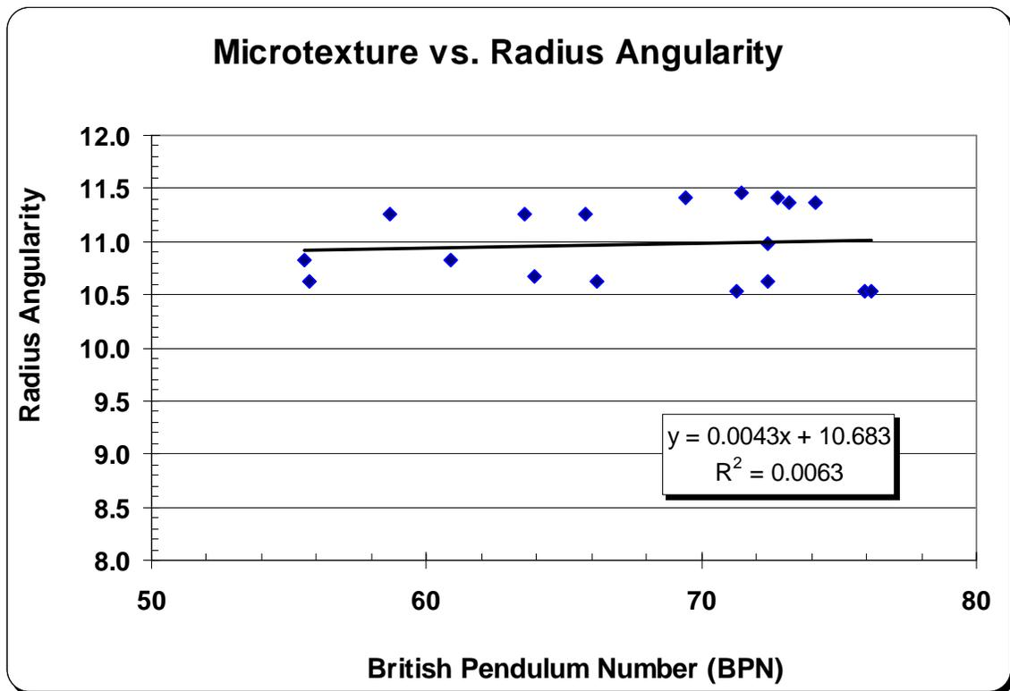
Figure 49. Relationship of Radius Angularity to Microtexture
