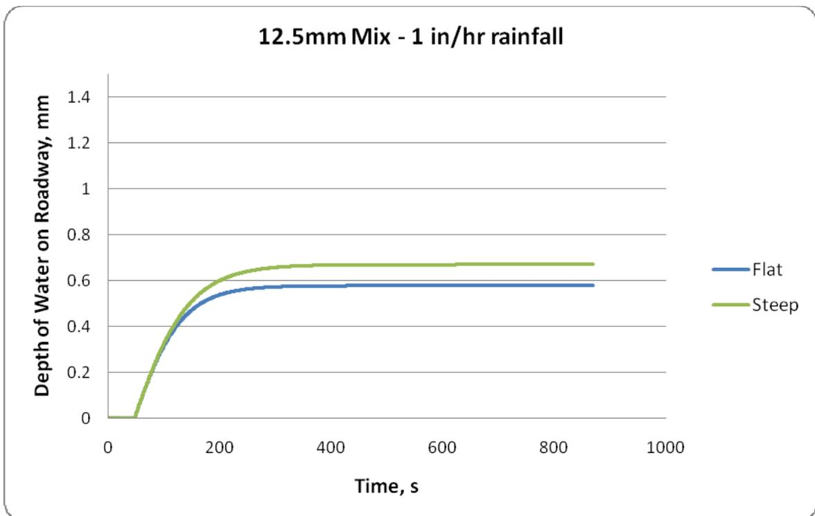
Figure 61. Net Depth of Water on Roadway vs. Time – 12.5mm Mix, Rainfall = 1 in/hr
