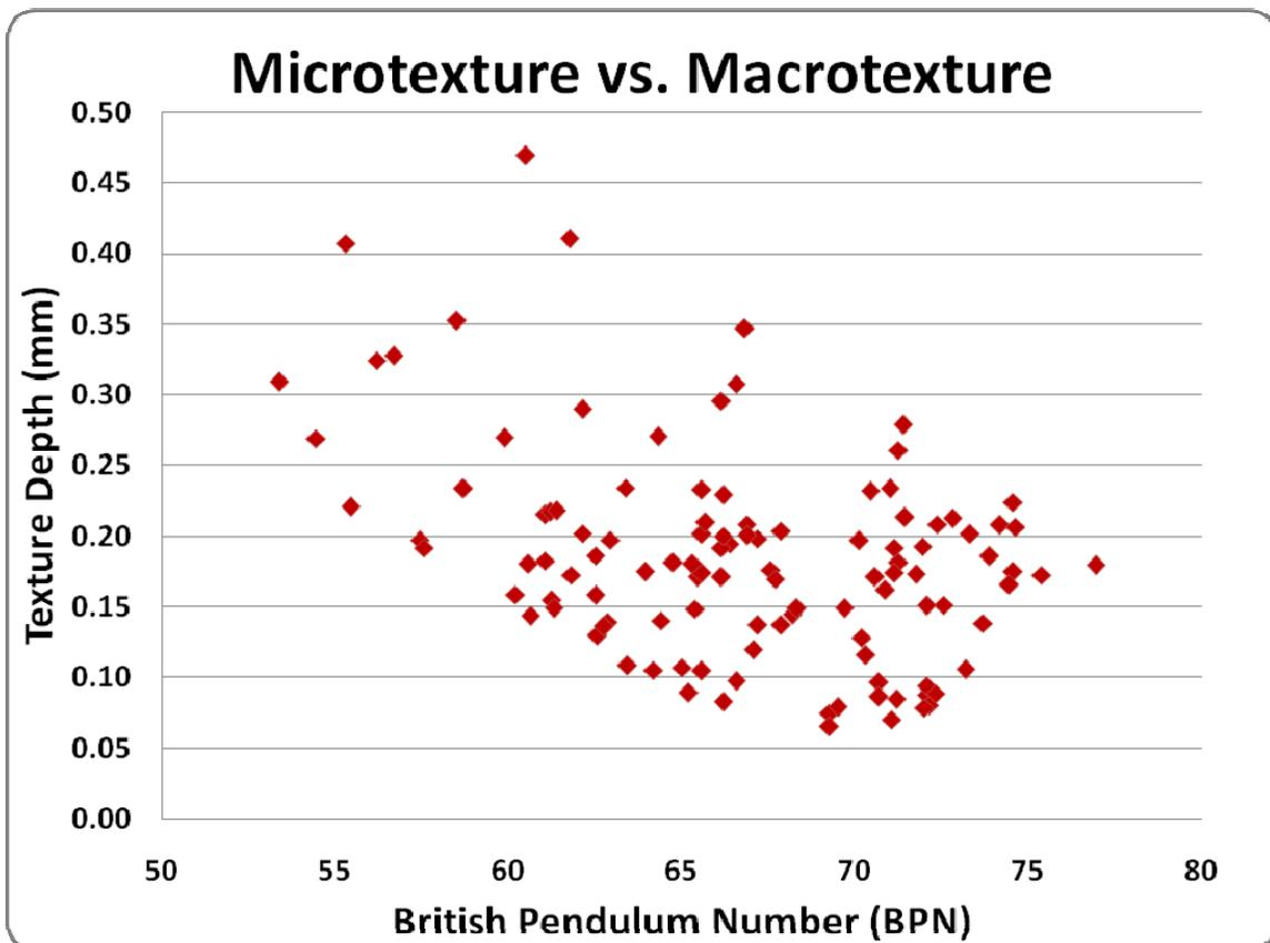
Figure 54. British pendulum Number vs. Texture depth for 4.75mm Mixes
