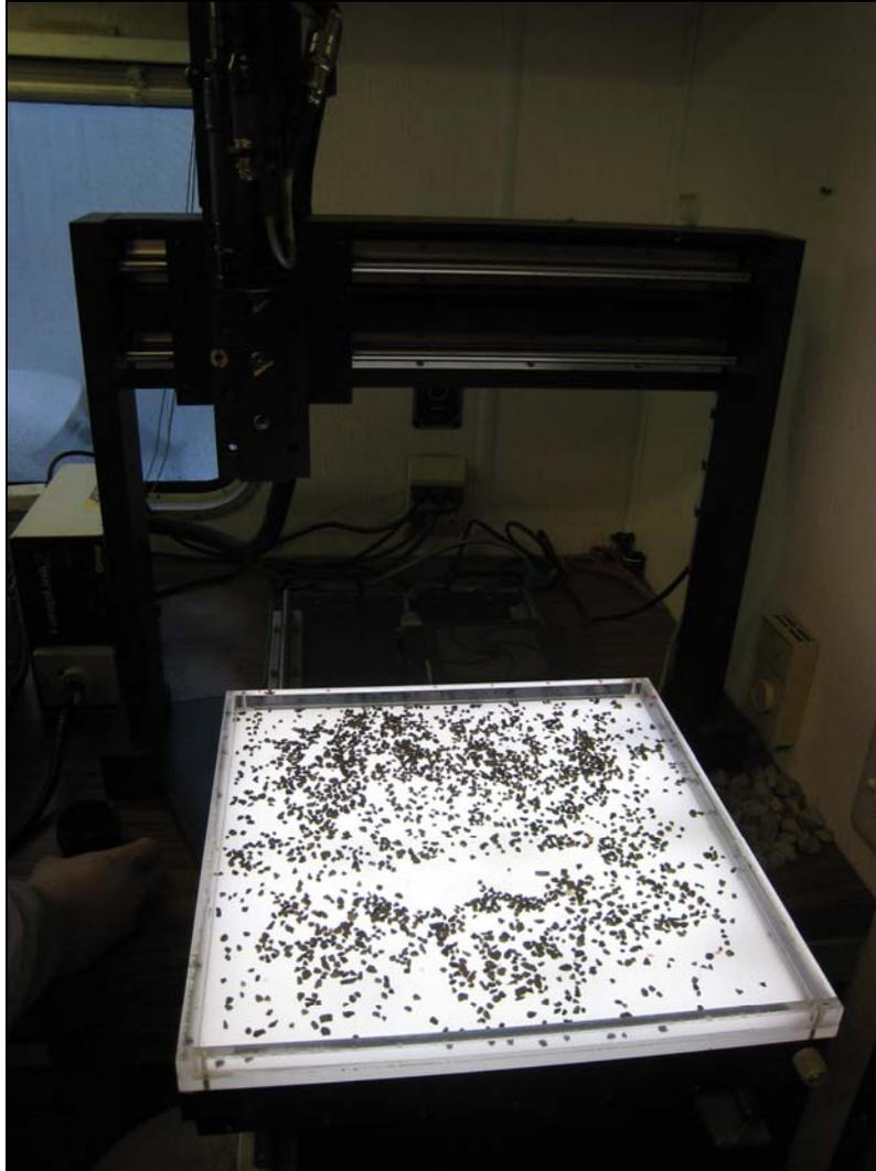
Figure 6. Aggregate Imaging System (AIMS)
