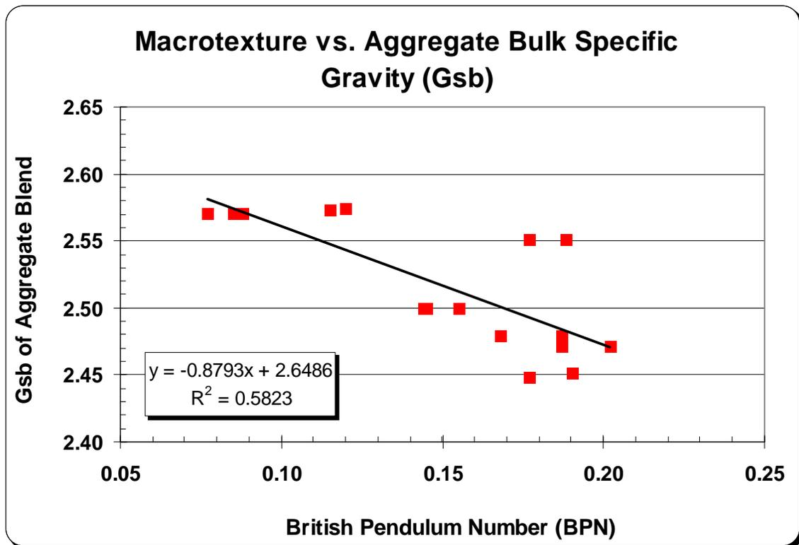
Figure 31. Relationship of Aggregate Bulk Specific Gravity to Macrottexture
