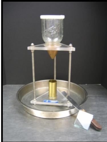
Figure 5. Fine Aggregate Angularity Apparatus
