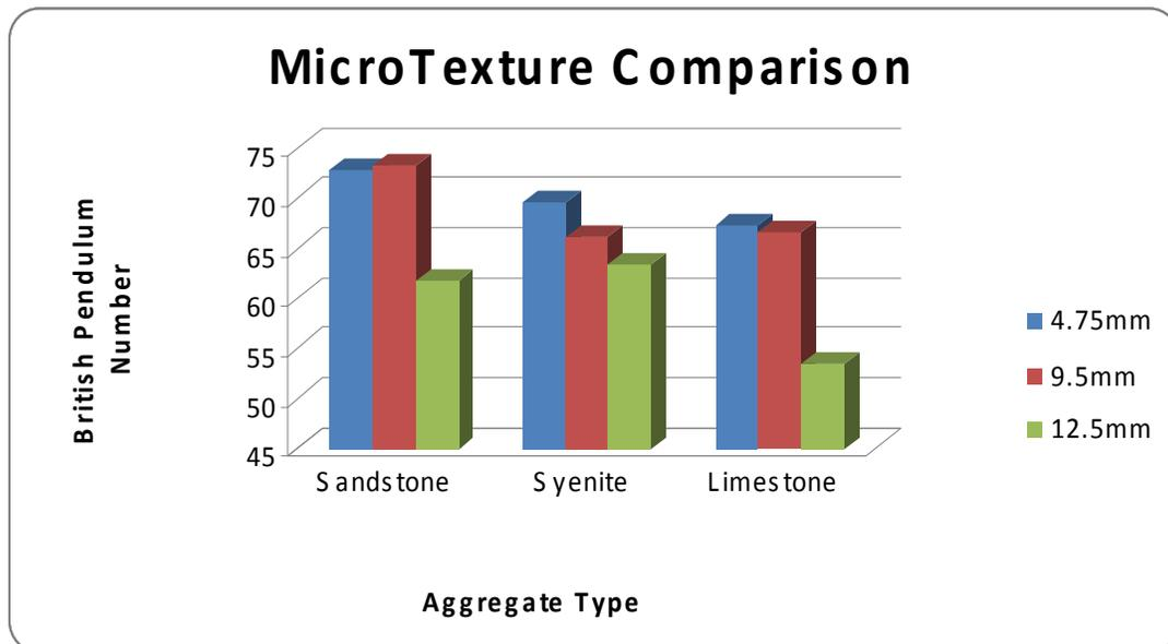
Figure 55. Effect of Nominal Maximum Aggregate Size on Microtexture
