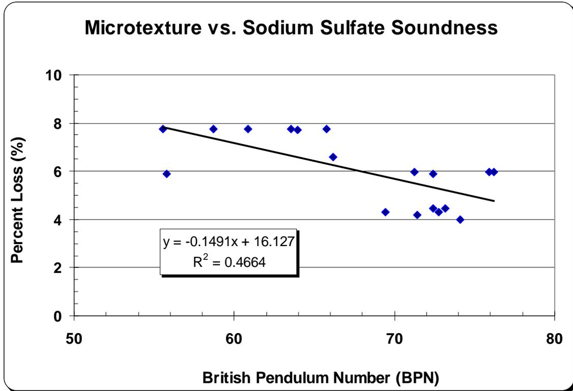
Figure 28. Relationship of Sodium Sulfate Soundness to Microtexture
