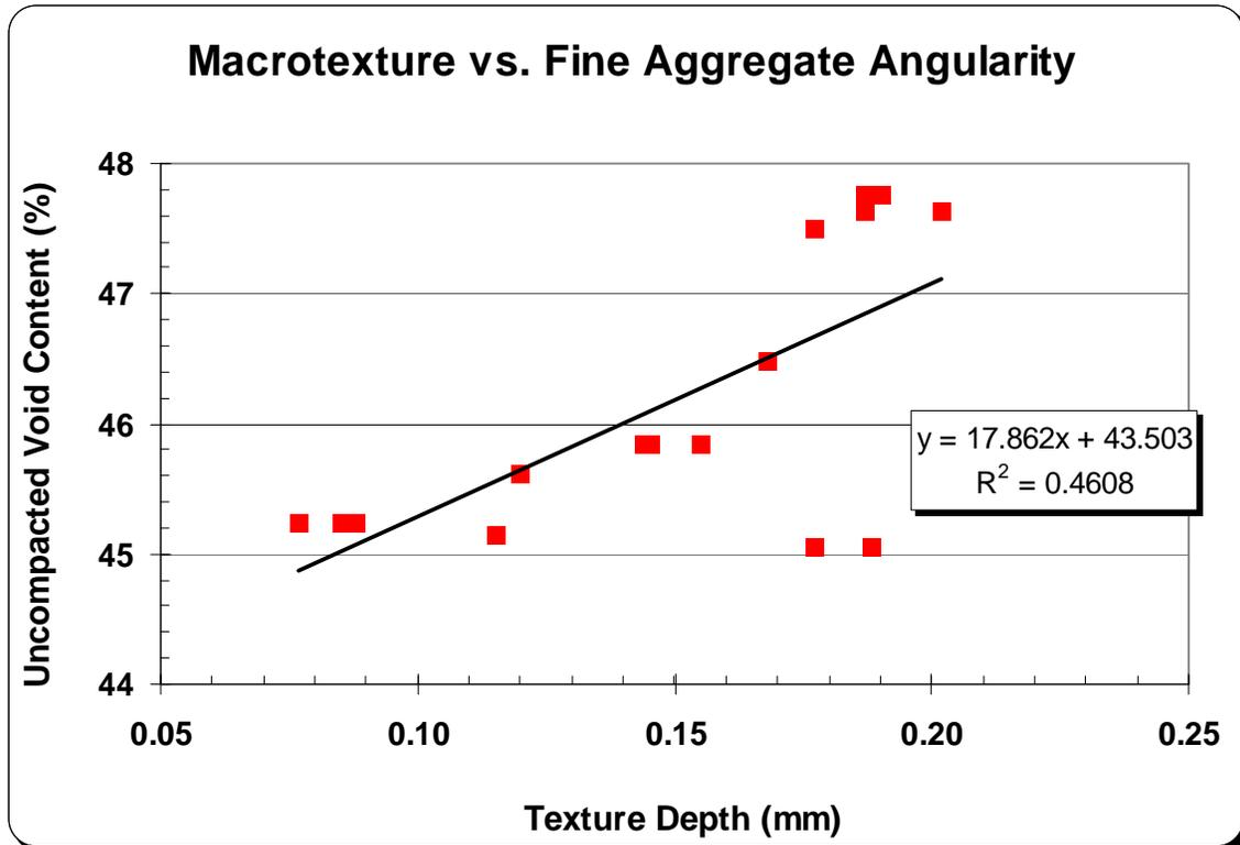
Figure 25. Relationship of Fine Aggregate Angularity to Macrotexture
