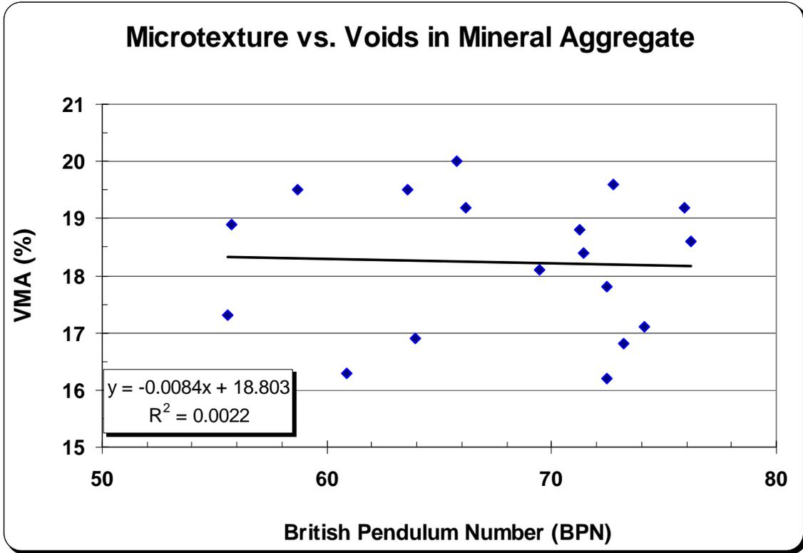
Figure 12. Relationship of Voids in Mineral Aggregate (VMA) to Microtexture
