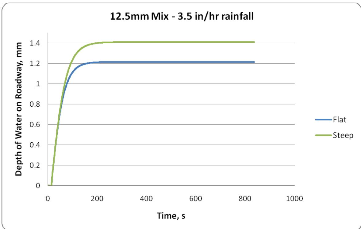
Figure 63. Net Depth of Water on Roadway vs. Time – 12.5mm Mix, Rainfall = 3.5 in/hr
