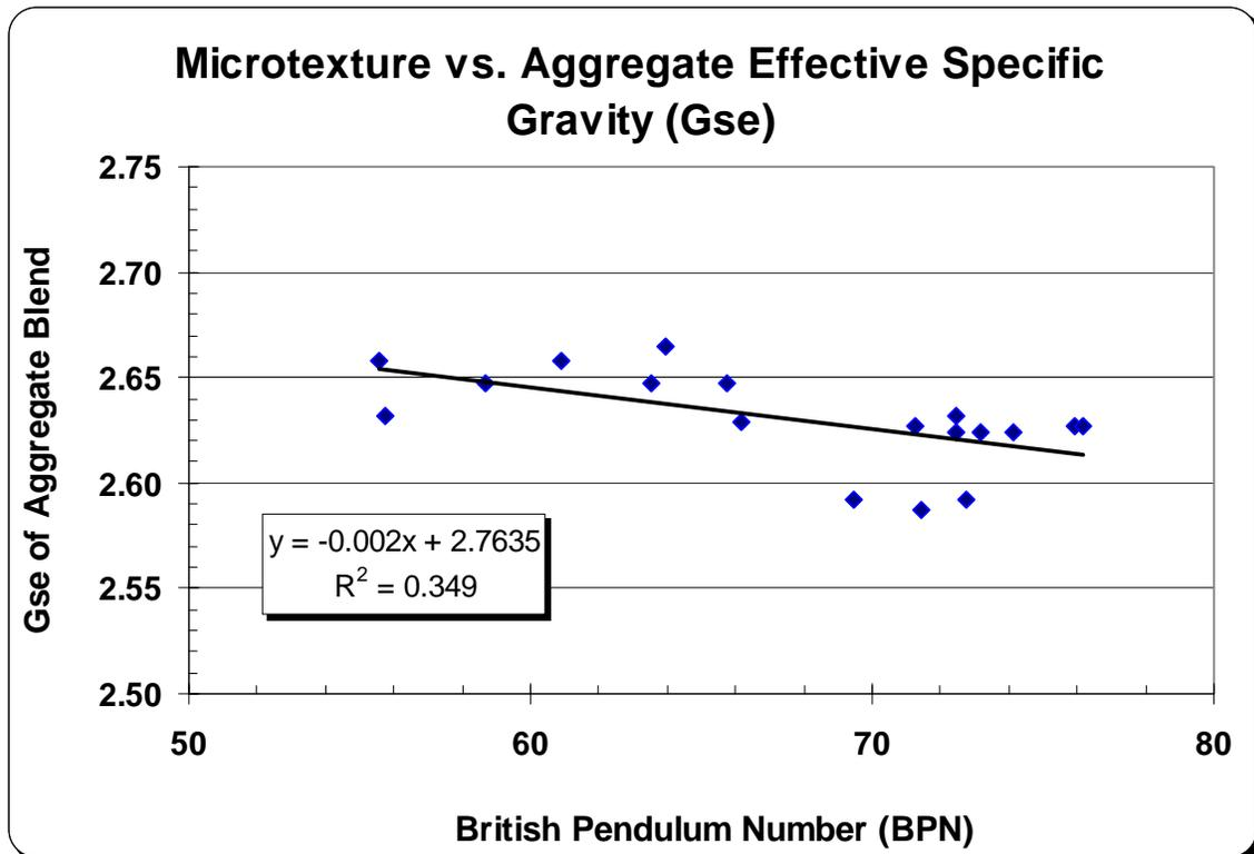
Figure 32. Relationship of Aggregate Effective Specific Gravity to Microtexture
