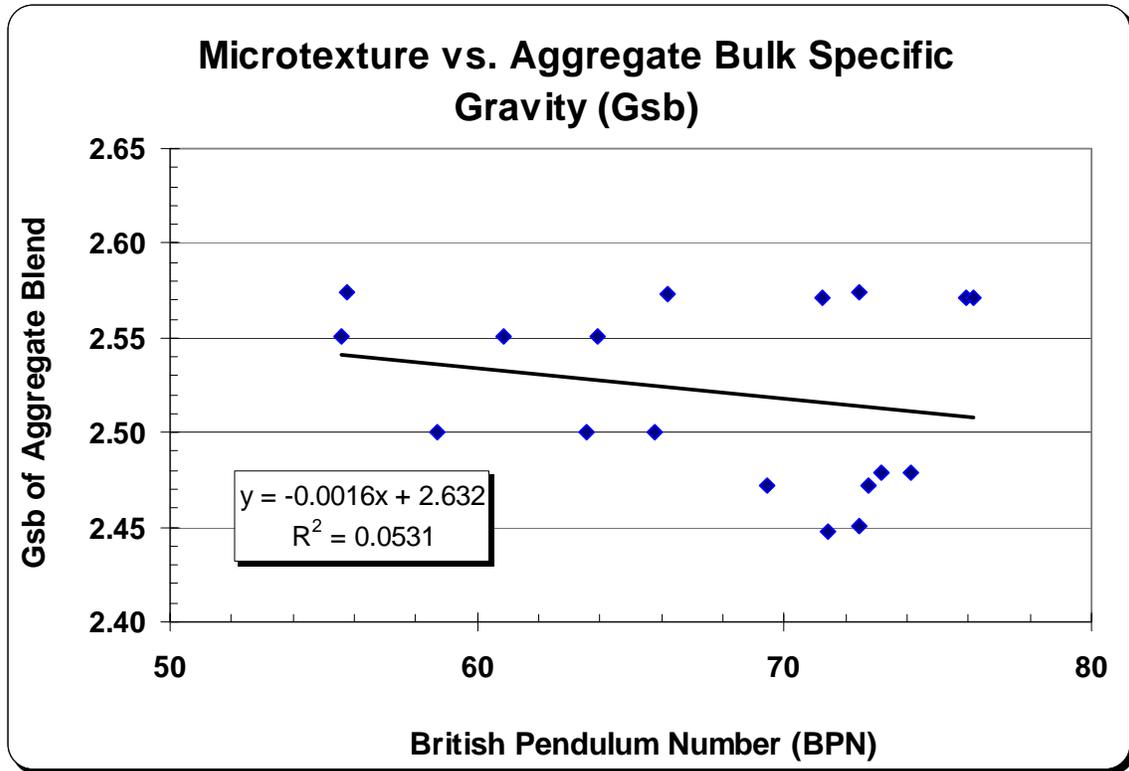
Figure 30. Relationship of Aggregate Bulk Specific Gravity to Microtexture
