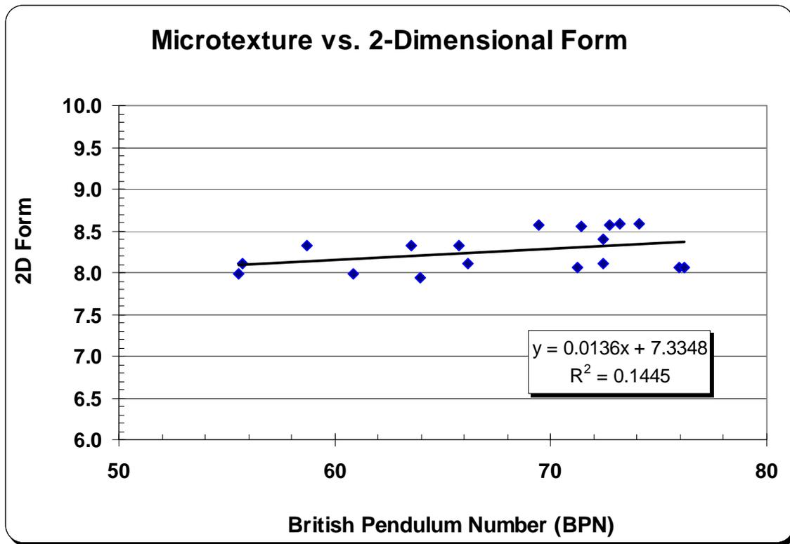
Figure 50. Relationship of Two-Dimensional Shape to Microtexture
