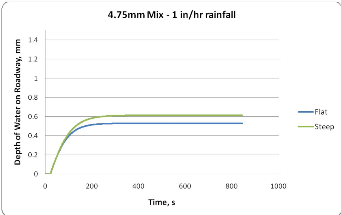
Figure 58. Net Depth of Water on Roadway vs. Time – 4.75mm Mix, Rainfall = 1 in/hr
