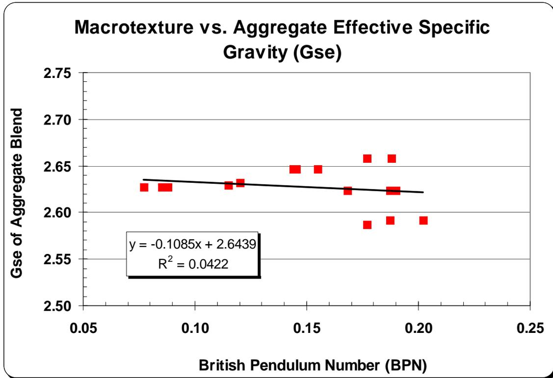
Figure 33. Relationship of Aggregate Effective Specific Gravity to Macrotexture
