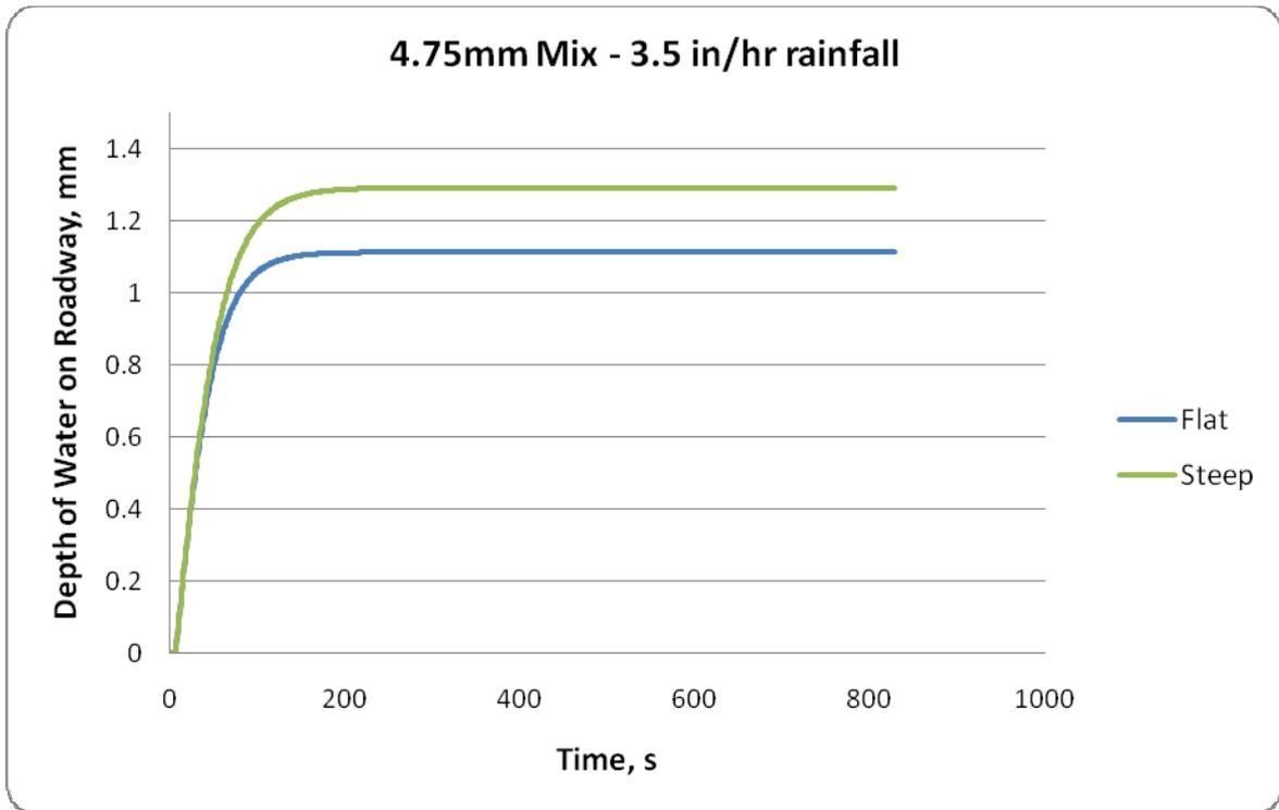
Figure 60. Net Depth of Water on Roadway vs. Time – 4.75mm Mix, Rainfall = 3.5 in/hr
