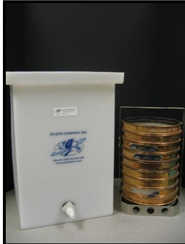
Figure 4. Sodium Sulfate Soundness Testing Equipment
