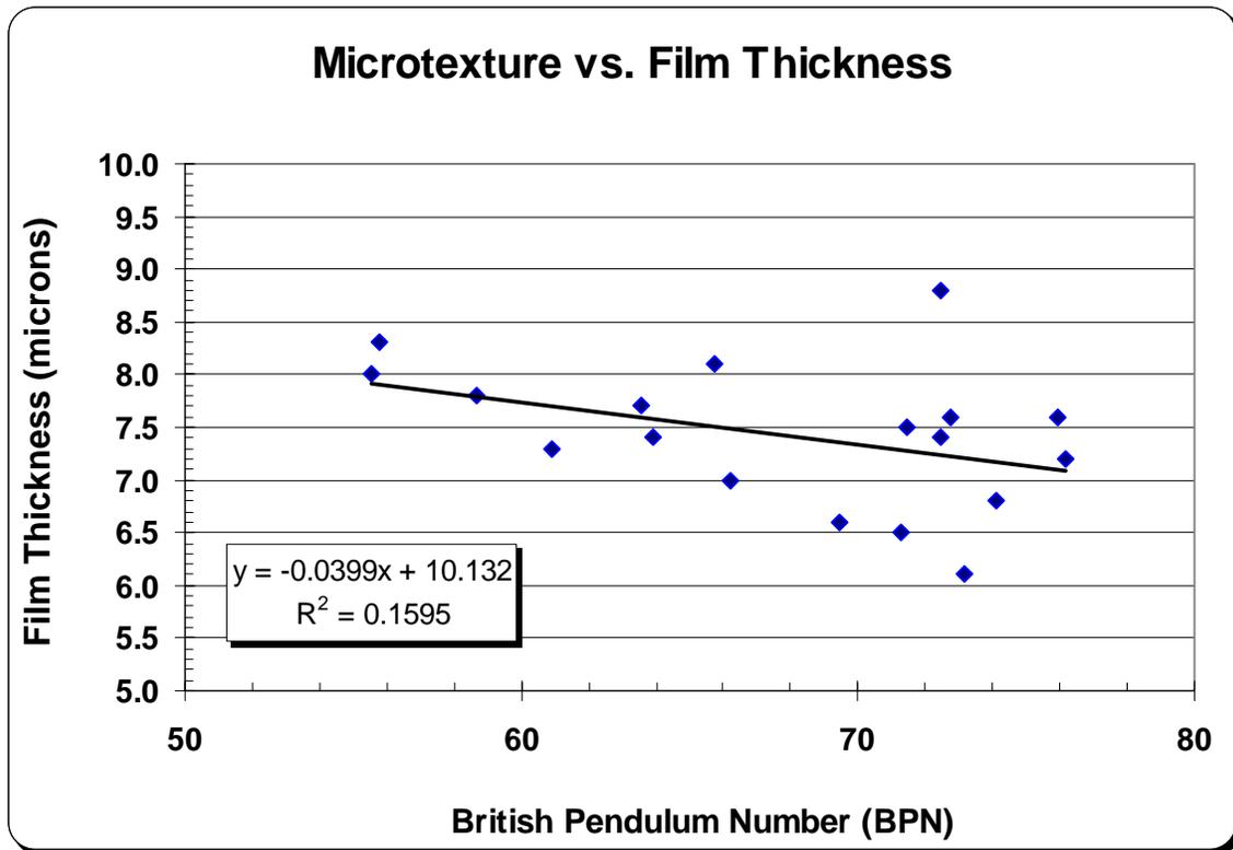
Figure 16. Relationship of Film Thickness to Microtexture
