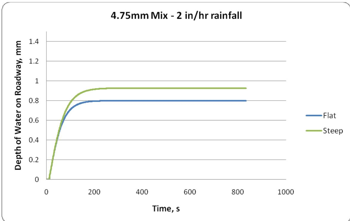
Figure 59. Net Depth of Water on Roadway vs. Time – 4.75mm Mix, Rainfall = 2 in/hr
