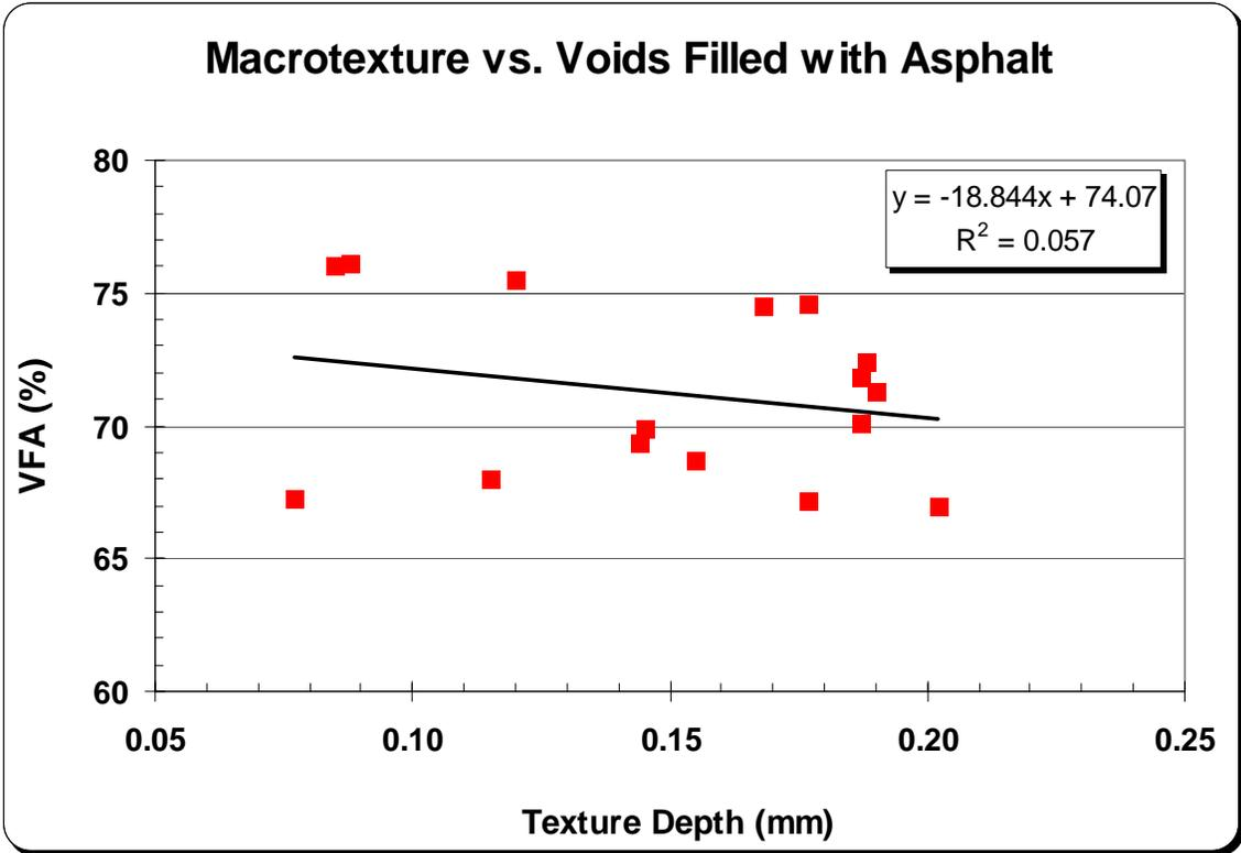
Figure 20. Relationship of Voids Filled with Asphalt (VFA) to Macrotexture
