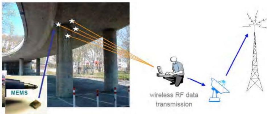
Figure 4 Diagram of wireless sensing of large structures using radio frequency transmission technique (after Grosse etc, 2004)
