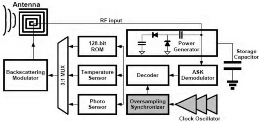
Figure 9 RFID sensor network (after Cho etc, 2005)
