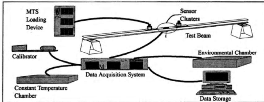
Figure 3 Bridge monitoring system Using MEMS Sensors (after Helmicki etc, 1995)
