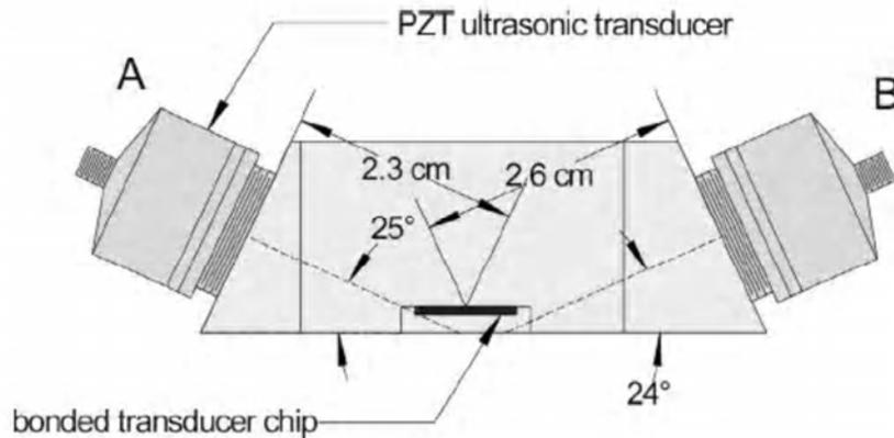
Figure 6 Drawing showing plexiglass test specimen with two off-axis locations for the emitting transducer (after Oppenheim etc, 2003 )
