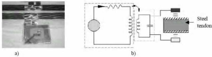
Figure 7 Wireless sensor system a) a wireless sensor for corrosion monitoring attached to a steel tendon;
