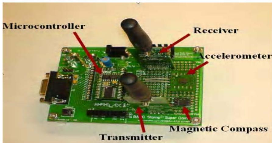
Figure 10 Prototype demo system (after Liu etc, 2006)
