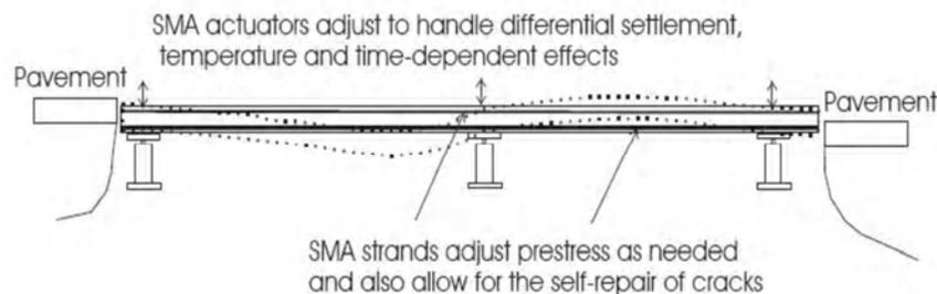
Figure 2 SMA smart material applied to bridge (after Cai etc 2004, Liu etc 2006 )
